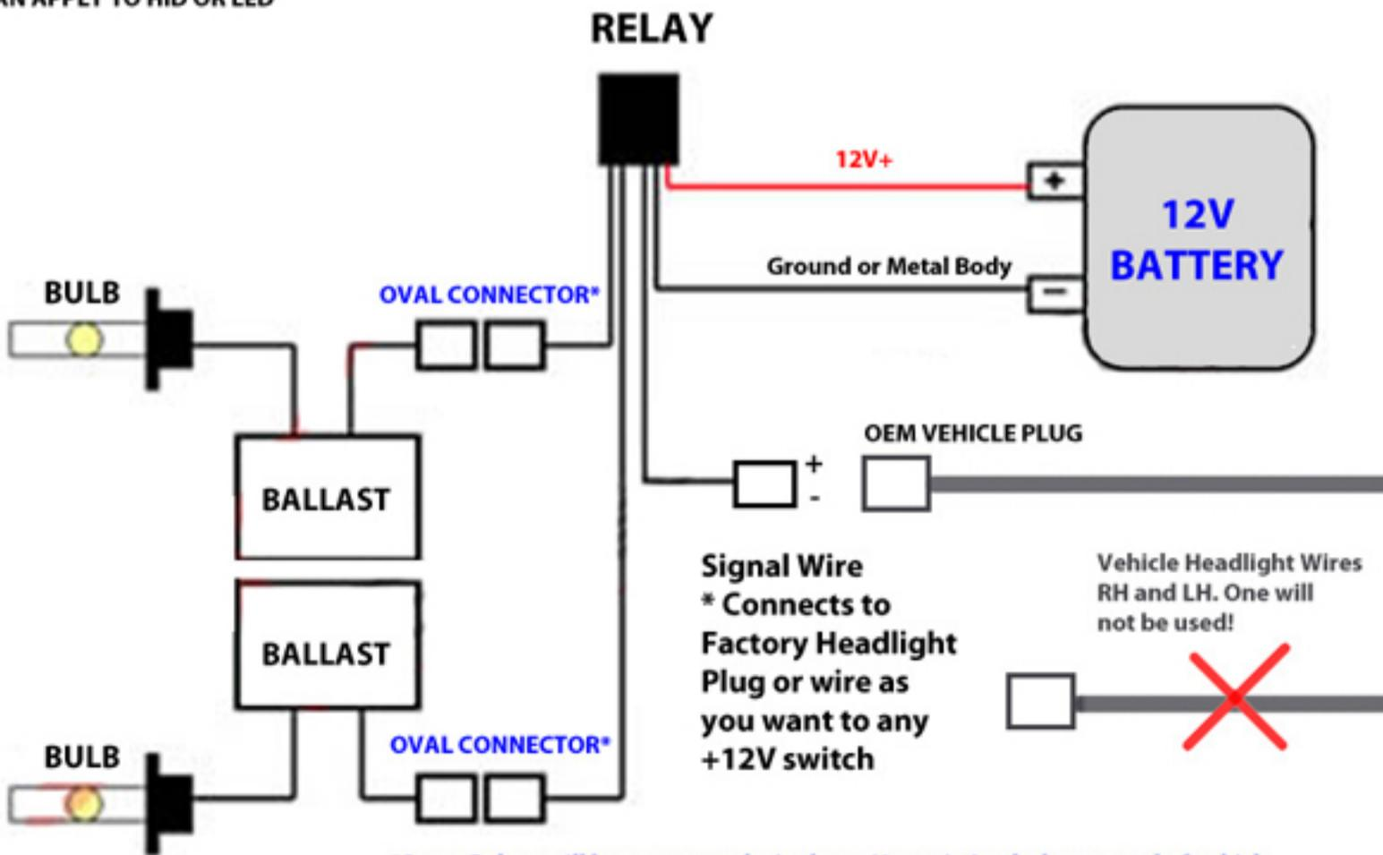
\*Some Relays will have a ground wire here. Use existing bolt on metal of vehicle.
